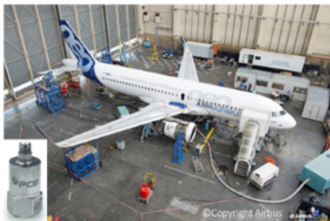
Floor vibration testing on an A320 Neo in Toulouse.
