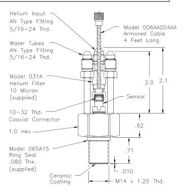
123 Series: Water- Cooled & Helium Bleed Rocket Motor, ICP® and Charge Sensors
