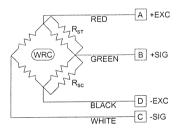
Figure 7 - Shunt Resistor Locations
