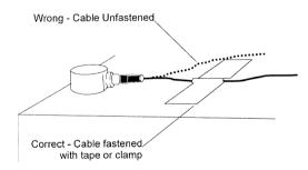
Figure 6 - Cable Strain Relief
